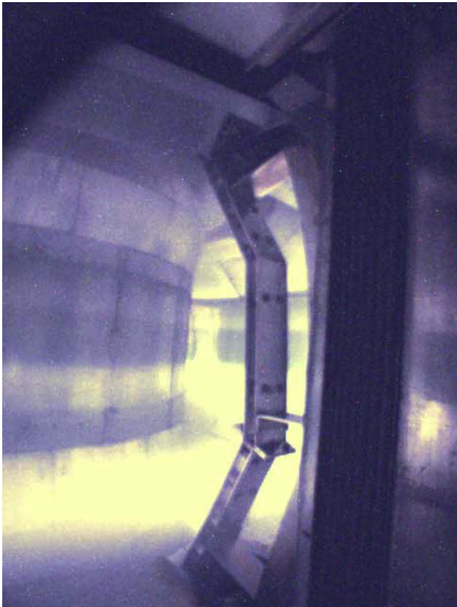
Fig. 2. The dedicated ICRF antenna for wall conditioning and a typical He-ICRF plasma, where the duty time of pulsed ICRF wave was set at 0.3 s on and 1.2 s off.
